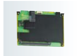
AJ-YA350AG HD/SD Input Board for AJ-HPX2000/HPX2100
